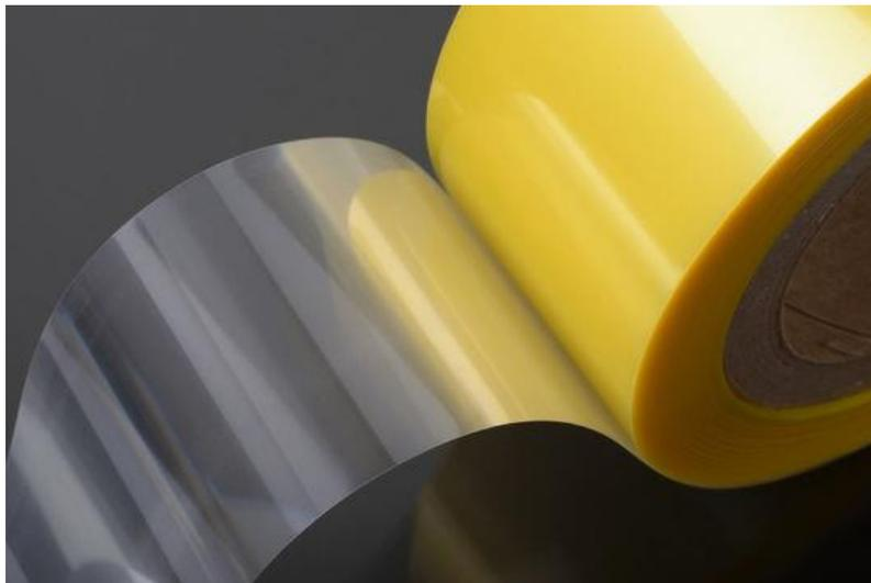
Microstructured surfaces off the roll: The structures are designed in a way to damage the cell envelopes of the microbes mechanically, to kill off pathogens (© Fraunhofer IPT)
